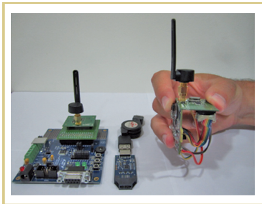
Figure 2. The portable transceiver iCube v0.1, developed for the course (on the right). It consists of a low-cost radio module interfaced to an MCU unit small-form-factor development kit. On the left are the AA-battery holder, the MCU toolstick USB programmer, and a radio module interfaced on an MCU development kit.
